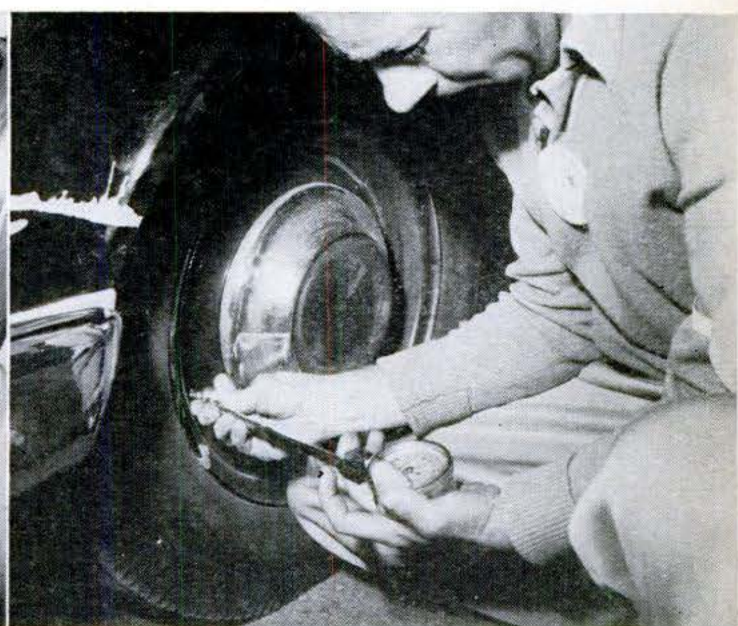
TIRE PRESSURES received careful attention before start of run. At its close, AAA officials checked pressures to make sure tires had not been extra-inflated to improve mileage.
